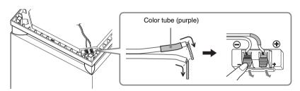
2 Thread the speaker cord through the gap along the side of the subwoofer, and secure it in the speaker cord holder.
